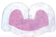
Open Barrel Connection Crimp
