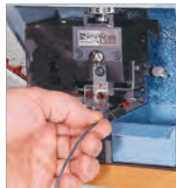
Next terminal or disconnect is automatically positioned under the dies
