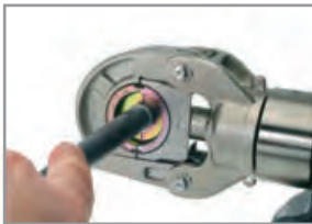
For an indent crimp the crimping order is reversed
