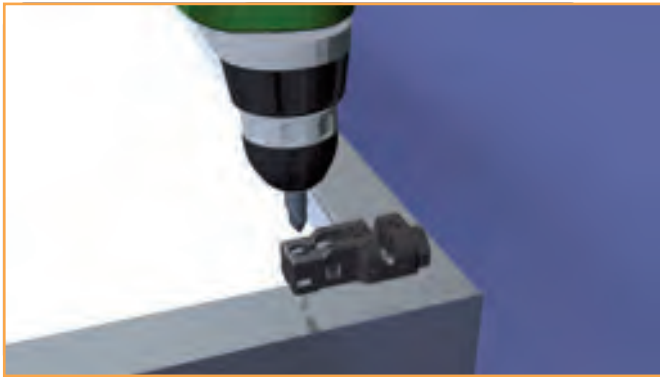
SOLFIT ® can be fixed quickly by drilling and tapping the chassis, using a screwdriver equipped with a PZ2 hexagon bit.
