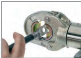
For an indent crimp the crimping order is reversed
